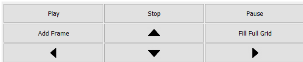
Figure 5: The Control Cluster has controls for shifting the node array in the indicated direction, as well as the ability to add a frame, color all nodes in the editor, and Play, Pause and Stop an animation
